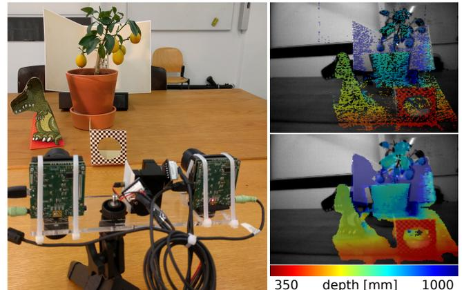
Fig. 1. **Left**: Stereo rig with two DVS and a MGDL in a scene. **Right**: Sparse and inpainted depth maps of the scene, reconstructed using our system.
